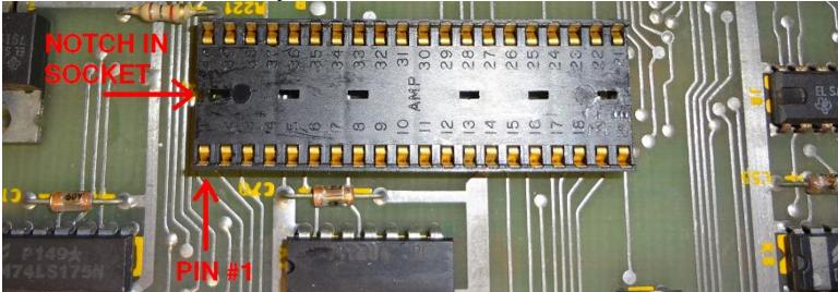
2) Install the new chip as shown with pin #1 matching pin #1 on socket. Verify all pins are aligned in
