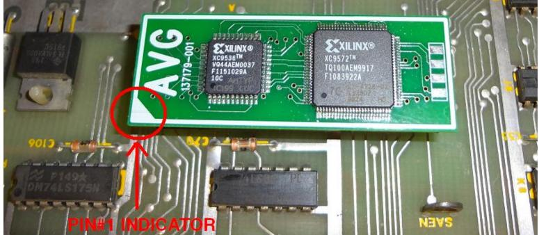
Note: The two Xilinx chips on the board can be easily damaged if the game board is stacked with other game boards. The chips have fine legs that can be easily bent if brushed against. To further protect the new chip hot glue or two part epoxy can be applied to the legs around the Xilinx chips. This will have no effect on the operation of the chip but will help protect the chip from outside handling/stacking of boards.
